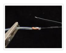
Now we can revisit the corona wires. Using the tip of the soldering iron, heat up the copper tape and melt a little solder on.
