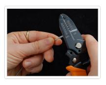
Next, we'll need to remove the outer coating. This is the hardest part of the process so don't be disappointed if it takes a few tries to get it right! Use the 20 AWG or 18 AWG slot and strip off the PVC coating about 1/2" (1 cm) away from the end.
