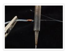
Now you have to heat up the heatshrink to get it to shrink. You can use a heat gun, hair dryer, hold it above a lighter (carefully!) or you can try 'rubbing' the non-solder part of your iron gently against the shrink.
