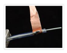
Now wrap the remaining tape around so that it covers and protects the solder joint.
