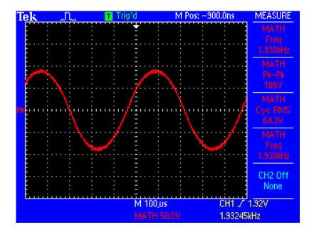
If you are comfortable using tools want to optimize your driver and wire, you can do so by 'modeling' your EL wire with a capacitor and resistor and plugging that in, then measuring the frequency across the RC with a multimeter or scope, just watch out you don't zap yourself!
