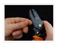
If you arent succeeding at getting the PVC off without damaging the wires, you can try not-quite-closing the cutters all the way (the image below is an exaggeration of how much to close it) and giving it a good yank.
