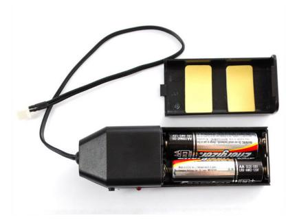
This pocket inverter can drive approximately 1 to 15 feet (0.3-5 meter) of 'classic' EL wire such as LyTec. Since we are using higher-brightness EL wire in the shop, it can only drive half as much, 1 to 7.5 feet (0.3 to 2.5 meter). We found that 2 meters gives a nice bright glow at good voltage and frequency. At 3 meters, its not as bright, it appears about the same as 'classic' EL.
