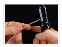
Start by cutting the wire to be as long as you want, and add an inch (or if you're starting out, a few inches) for the wire connection. Remember, its very easy to make the wire shorter but hard to make it longer!
