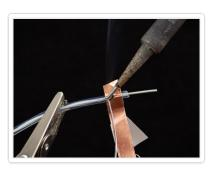
Heat up your soldering iron to 650 degrees F and make sure its hot by melting solder onto the tip, it should melt easily.now press the tip of the iron to the two wires and copper tape and quickly dap some solder in.then remove the iron. This should not take more than a second or two or the EL wire casing will melt.
