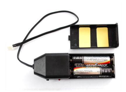
The voltage should be between 50-120V AC RMS (150V-360V peak-to-peak). Higher voltages result in a brighter display (but lower overall wire-life).
